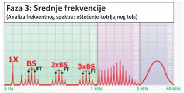
Stage Three: Ball or roller fault (inner race rotating)
